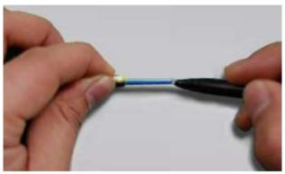
4.Mark the 22mm long point on the 900 buffer  $\mu$ m using a ruler in the polythene bag.
