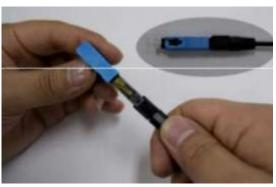
10. Flip the housing ledge down and attach it to the body.
