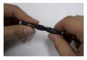
A. Take out the casing and then separate it by turning the screw cap
