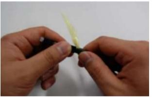
9. Take the boot cover down, connect the screw cap with the boot by twisting it, and make the liner and strength member fixed.
