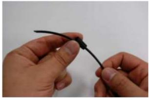
2. Insert the screw cap onto the optical cable.
